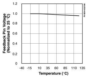
Figure 5. Feedback Pin Voltage vs. Temperature.
