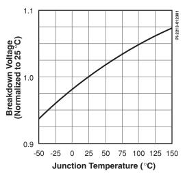
Figure 6. Breakdown vs. Temperature.
