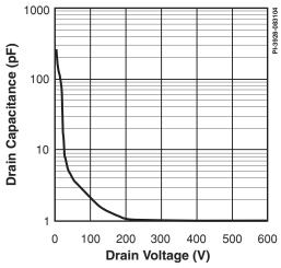
Figure 9.  $C_{\rm OSS}$  vs. Drain Voltage.
