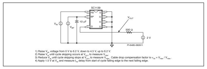
Figure 10. Test Set-up for FEEDBACK Pin Measurements.
