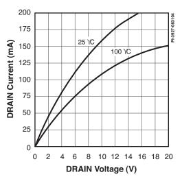
Figure 8. Output Characteristics.
