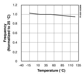
Figure 4. Output Frequency vs. Temperature.
