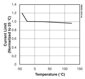
Figure 7. Current Limit vs. Temperature.
