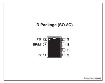
Figure 3. Pin Configuration.
