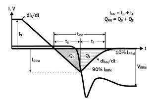
Figure 17. Diode Recovery Waveform
