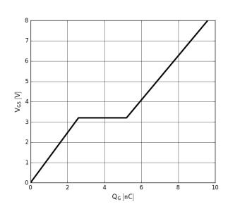
Figure 8. Typical Gate Charge  $I_{DS}$ =4A,  $V_{DS}$ =400V
