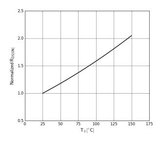
Figure 4. Normalized On-resistance  $I_D{=}16A,\,V_{GS}{=}10V$
