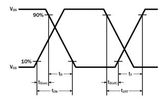
Figure 15. Switching Time Waveform
