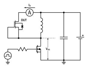
Figure 16. Diode Characteristics Test Circuit
