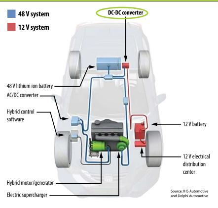
Figure 1. Representation of 48 V mild hybrid system
