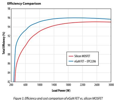
in a 48 V to 12 V , 3 kW system
