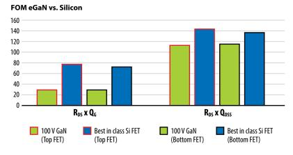
Figure 4. Figure of Merit (FOM) eGaN FET vs. Silicon MOSFET
