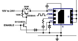
Fig. 22. Standby mode V<sub>CC</sub> cut-off circuit
