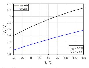
Fig. 7.  $V_{PWMH}$  and  $V_{PWML}$  vs. junction temperature( $T_{J}$ )
