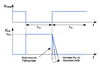
Fig. 23. Turn-on dV/dt slew rate control
