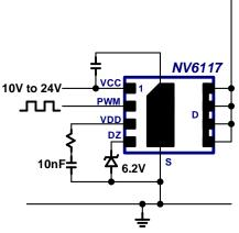
Fig. 18. Quick start-up circuit
