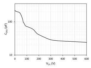
Fig. 9. Output capacitance  $(C_{OSS})$  vs. drain-to-source voltage  $(V_{DS})$
