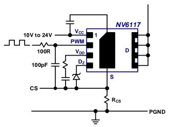
Fig. 24. Current sensing circuit
