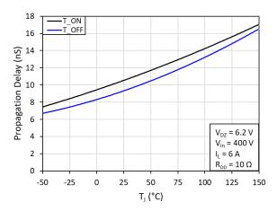
Fig. 14. Propagation delay  $(T_{ON} \text{ and } T_{OFF})$  vs. junction temperature  $(T_I)$
