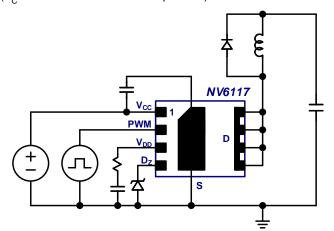
Fig. 1. Inductive switching circuit
