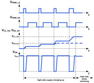
Fig. 20. ACF half-bridge start-up timing diagram
