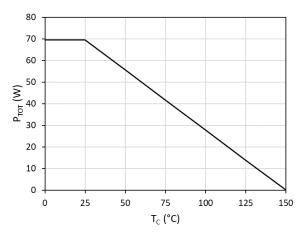
Fig. 16. Power dissipation ( $P_{TOT}$ ) vs. case temperature ( $T_{\rm C}$ )
