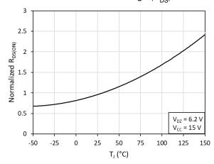
Fig. 8. Normalized on-resistance  $(R_{DS(ON)})$  vs. junction temperature  $(T_i)$
