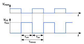
Fig. 21. Normal operating mode timing diagram
