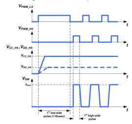
Fig. 19. LLC half-bridge start-up timing diagram
