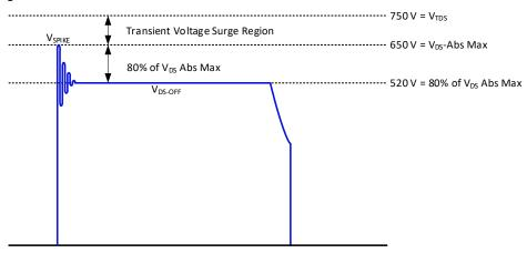
Fig. 28. QR flyback drain-to-source voltage stress diagram
