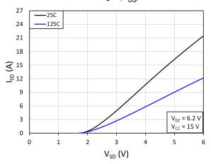
Fig. 5. Source-to-drain reverse conduction voltage
