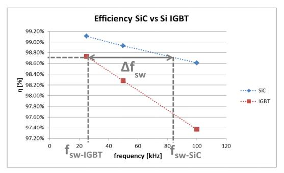
Fig.2. Efficiency vs switching frequency in ST 5kW Boost converter reference design
