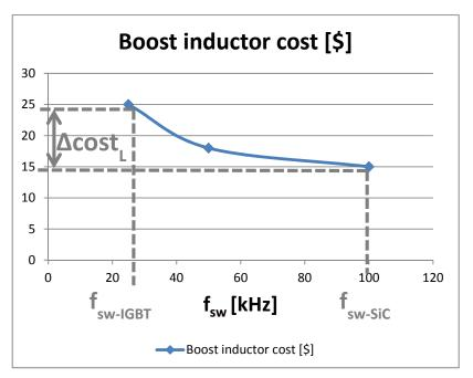
Fig.3. Typical cost of the inductor vs switching frequency
