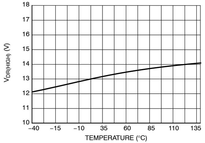
Figure 22. Drive Voltage V<sub>DRV(HIGH)</sub> vs Temperature
