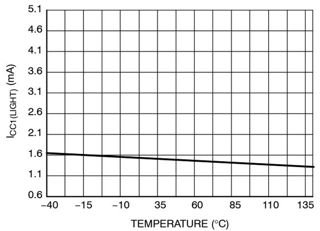
Figure 18. I<sub>CC1(LIGHT)</sub> vs Temperature
