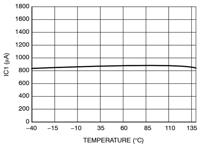
Figure 31. IC<sub>1</sub> Startup Current vs. Temperature
