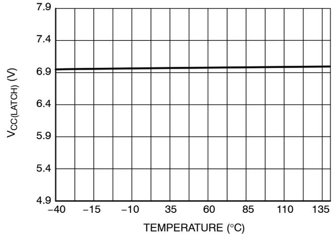
Figure 14. V<sub>CC(LATCH)</sub> vs Temperature
