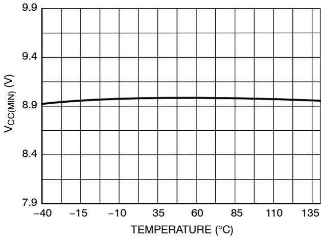
Figure 13. V<sub>CC(MIN)</sub> Voltage vs Temperature
