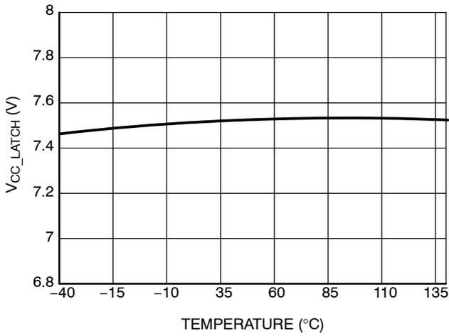
Figure 3. V<sub>CC\_LATCH</sub> vs. Temperature
