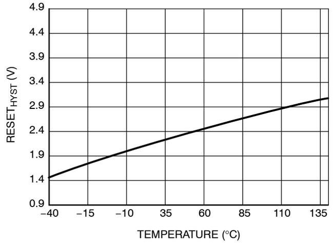
Figure 16. V<sub>CC(LATCH)</sub>-V<sub>CC\_HYST</sub> vs Temperature
