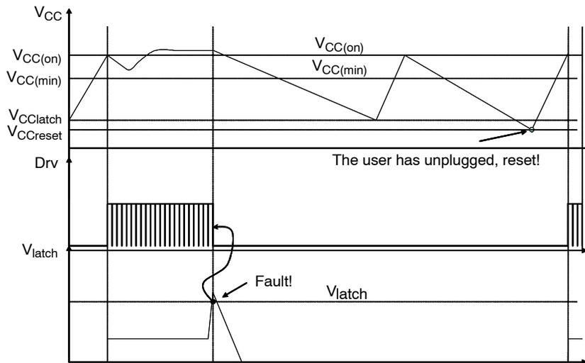
**Figure 40. The Part is Reset when V<sub>CC</sub> Reaches 5 V or when BO Senses the Bulk Capacitor Voltage is Back to Normal**
