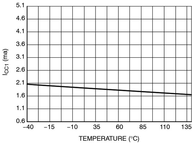
Figure 17. I<sub>CC1</sub> vs Temperature
