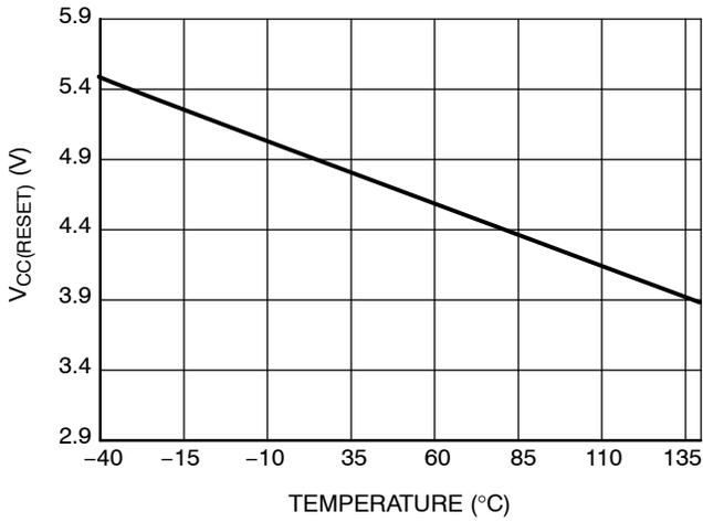
Figure 15. V<sub>CC(RESET)</sub> vs Temperature
