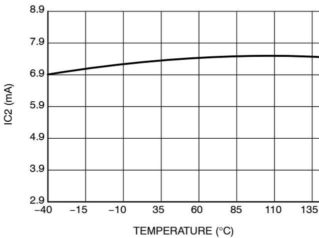
Figure 30. IC<sub>2</sub> Startup Current vs. Temperature
