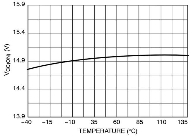
Figure 12. V<sub>CC(ON)</sub> Voltage vs Temperature
