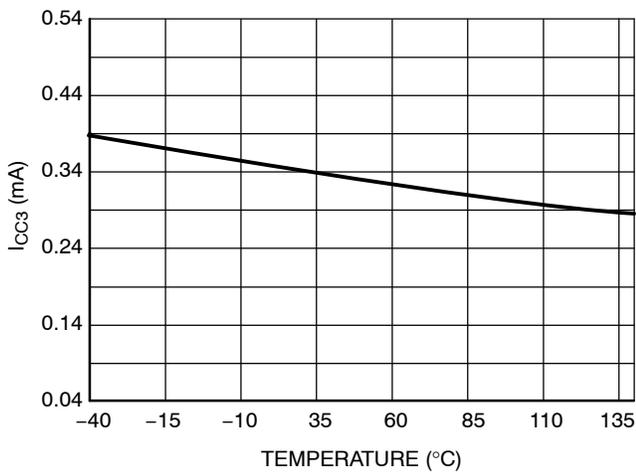
Figure 19. I<sub>CC3</sub> vs Temperature
