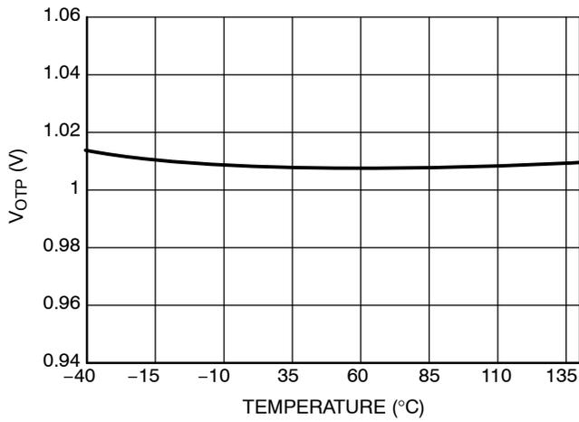
Figure 27. V<sub>OTP</sub> Voltage vs. Temperature
