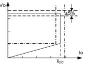
Figure.1. Typical CC/CV Curve
