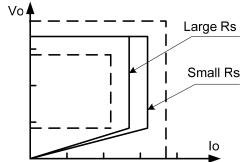
Figure.3. Adjustable output power by changing Rs
