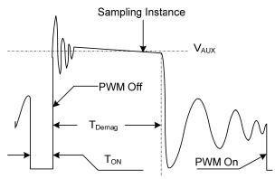
Figure.2. Auxiliary voltage waveform
