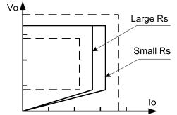
Figure.3. Adjustable output power by changing Rs
