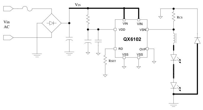
Figure 1: Typical Application Circuit Diagram 1 of QX6102 (without output capacitor)
