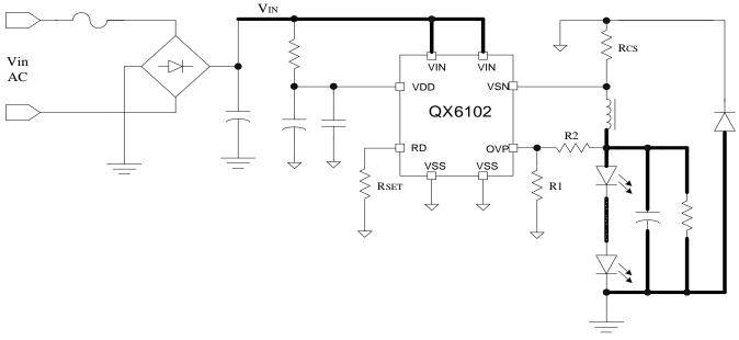
Figure 2: Typical Application Circuit Diagram 2 of QX6102 (with output capacitor)
