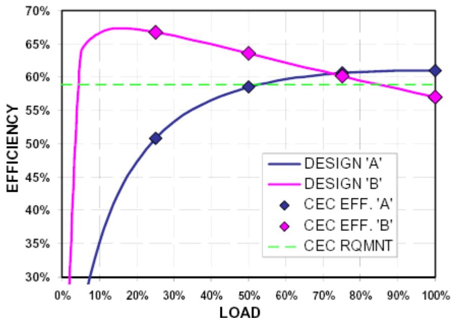
*TinySwitch-II* circuits can achieve such high light load efficiency because *EcoSmart®* technology automatically reduces the frequency of operation at light loads as a result of the On/Off regulation system, only switching to provide a power pulse when required. Consequently, switching losses are reduced to a minimum.
