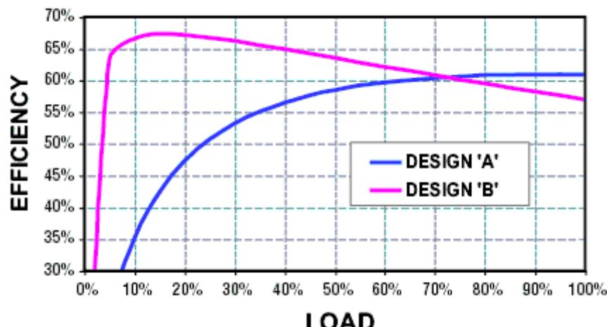
For your 3 W, 5 V CEC-compliant charger, two designs points, 'A' and 'B', are being considered, with efficiency versus load characteristics as shown in the figure. Which would be a better choice to meet the CEC requirements and why?
