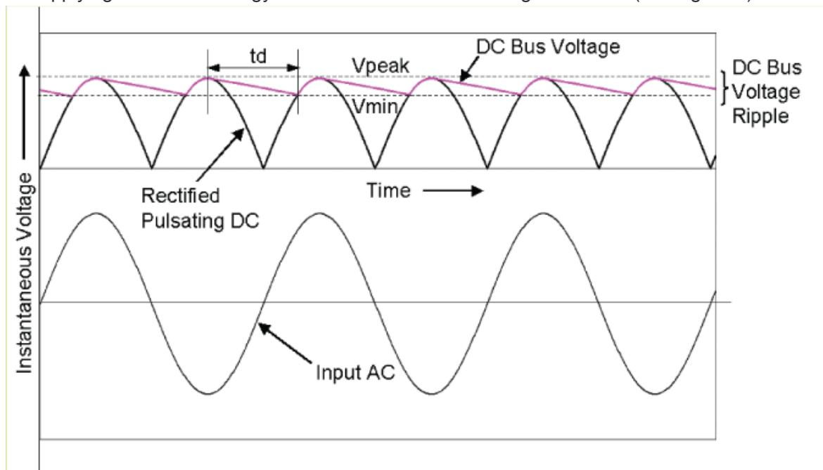
**Figure 2. Capacitive filter for full wave rectifier**
