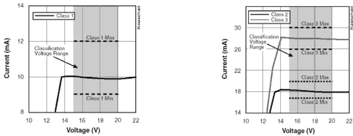
**Figure 4** - Class 1 to Class 3 - PoE Detection and Classification Specifications.
