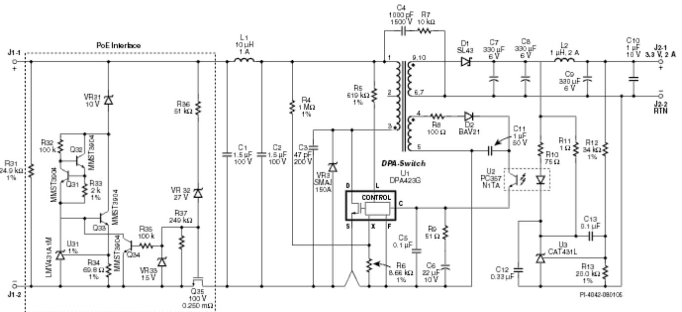
Figure 3 – PoE Class 2 DC-DC Converter Using DPA423G.
