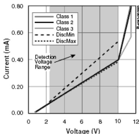
(a) Detection Current vs. Input Voltage
