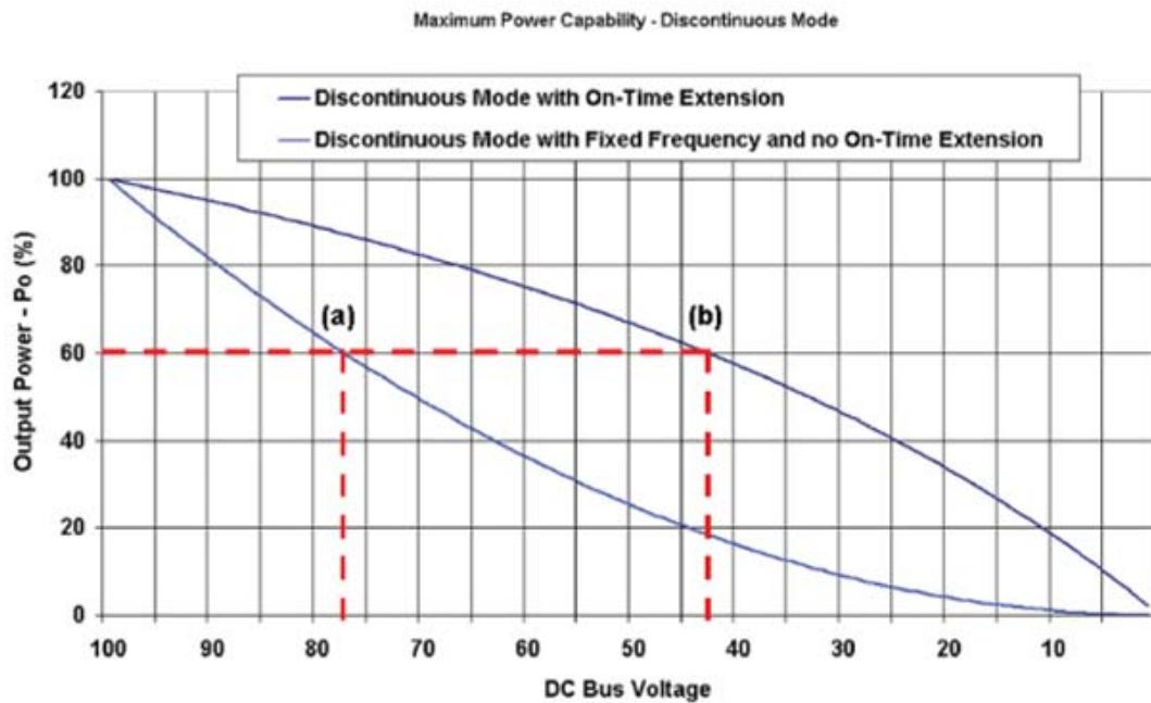
**Figure 5. Relation between DC Bus Voltage drop and power delivery capability of Flyback power supplies with and without on time extension. At 60% load regulation is lost at 77 V (a) without on-time extension and 43 V (b) with on-time extension.**
