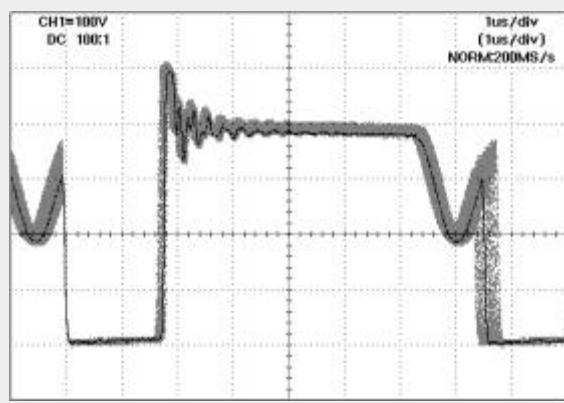
Figure 5 - *TOPSwitch-GX Jitter Waveform*
