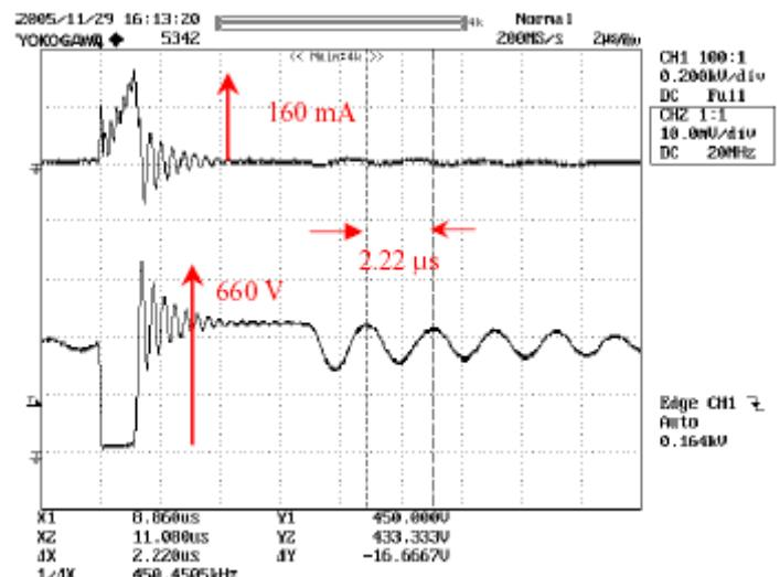
Drain Voltage and Current (200 V, 100 mA, 2  $\mu$ s/div.)
