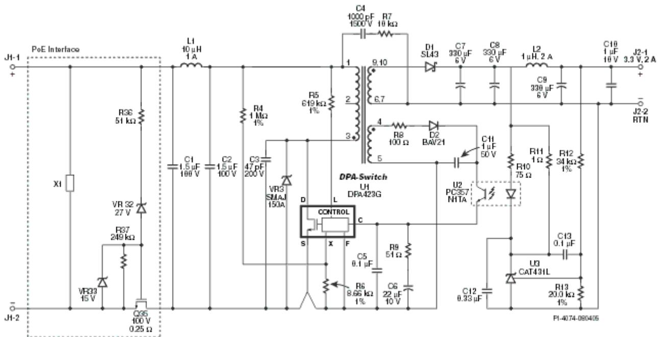
**Figure 1 – PoE Class 0 DC-DC Converter using DPA423G.**
