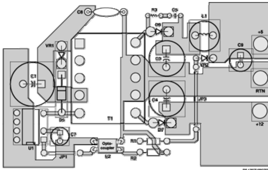
Figure 4: Improved layout for partial circuit shown in Figure 3.
