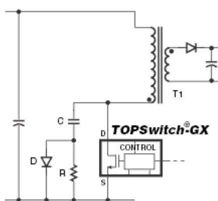
c) A circuit that can be used either to clamp the drain voltage or to limit the rate of rise of the drain voltage at turn off
