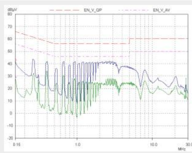
Figure 7 - *TOPSwitch-GX* (132 kHz) with jitter Conducted EMI versus Frequency
