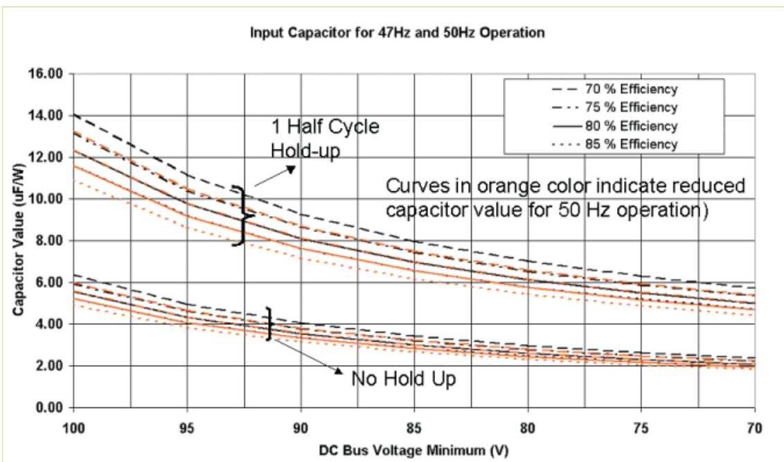
**Figure 4. Relative comparison of required capacitor value for 47Hz and 50Hz operation. Notice the slight reduction for a 50Hz only design**
