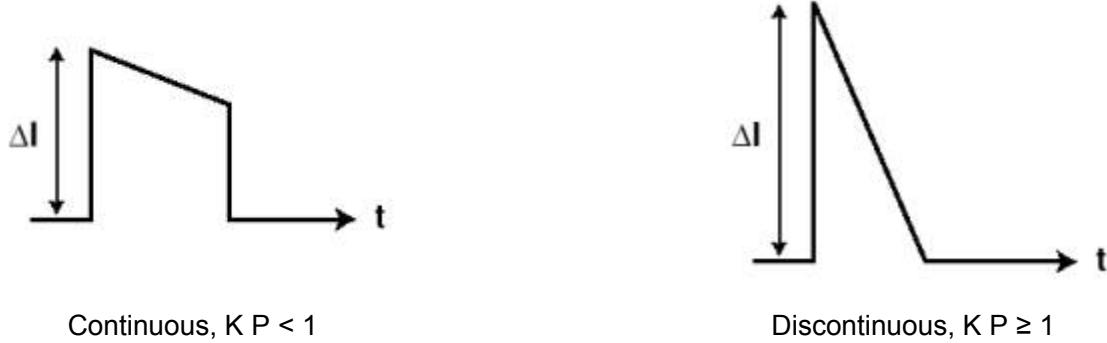
**Figure 8b** Example of secondary current waveform
