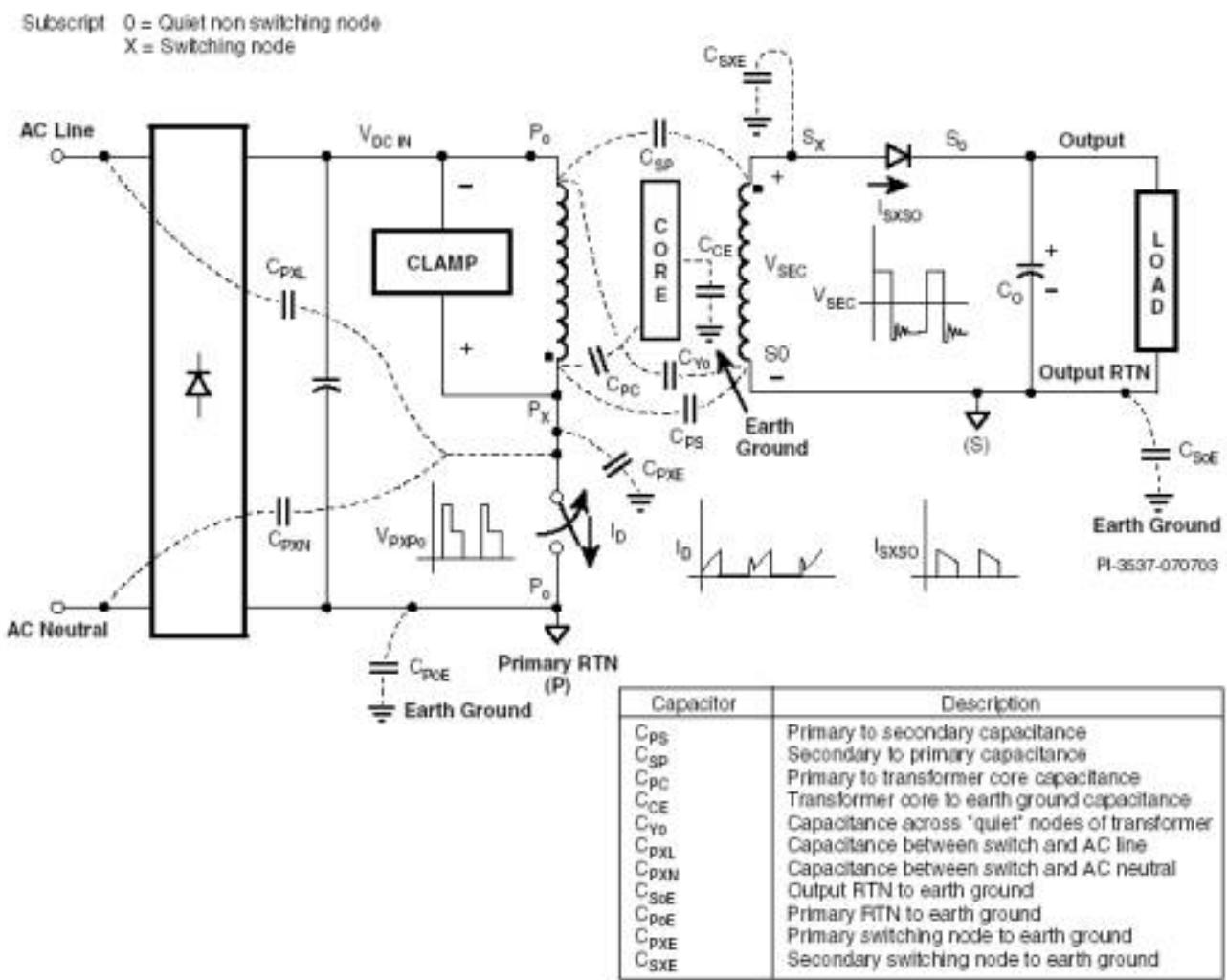
Figure 8 - EMI Sources and Coupling
