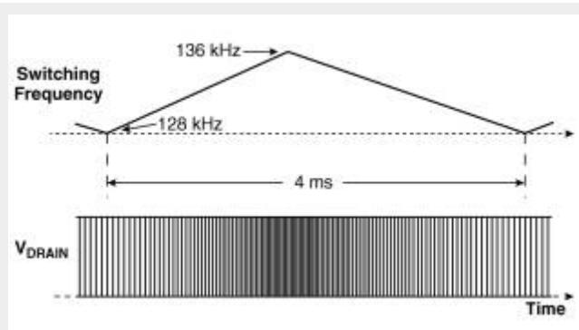
Figure 3 - *TOPSwitch®-GX Jitter Frequency*
