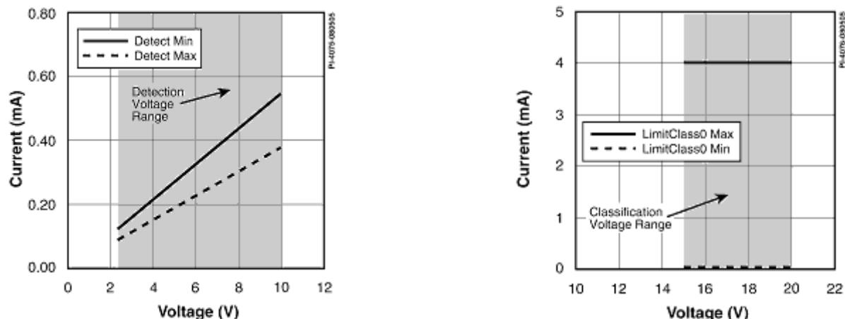
**Figure 2 – Class 0 - PoE Detection and Classification Specifications.**
