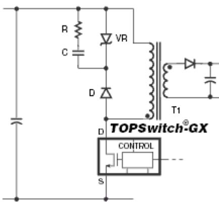
Circuit ‘C’ is a well controlled clamp circuit that accurately limits the maximum Drain voltage, while also giving the lowest no-load consumption and best efficiency.
