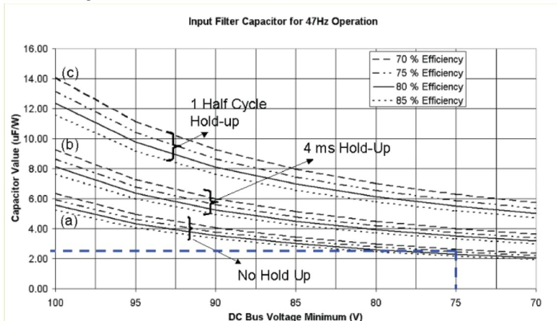
**Figure 3. Capacitor selection curves for 47Hz frequency universal input application. (a) No hold up requirement, (b) 4ms hold up requirement and (c) hold up of one half cycle of supply frequency)**
