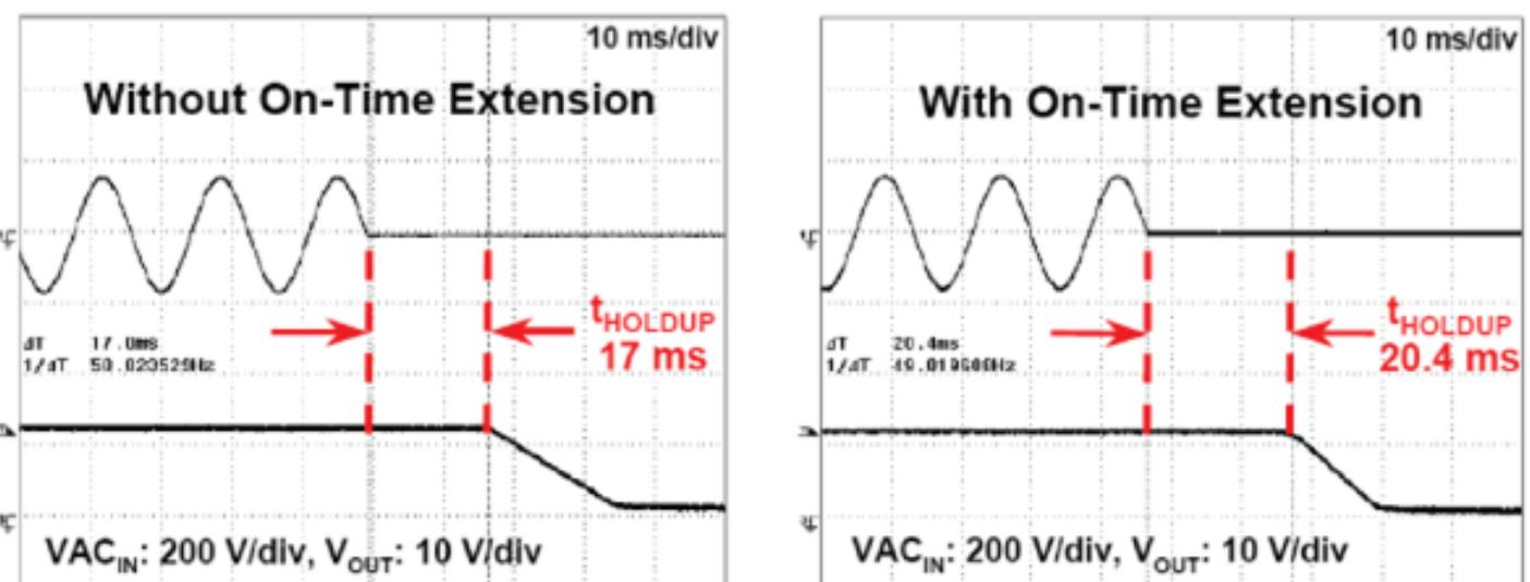
**Figure 6. Improvement in hold up time with on time extension**
