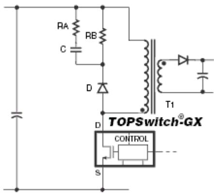
The lowest cost approach to dissipating leakage inductance energy is to provide a diode clamp to an RC network, as in circuit 'B'. Such circuits are known as 'Resistor-Capacitor-Diode' (RCD) clamps.
