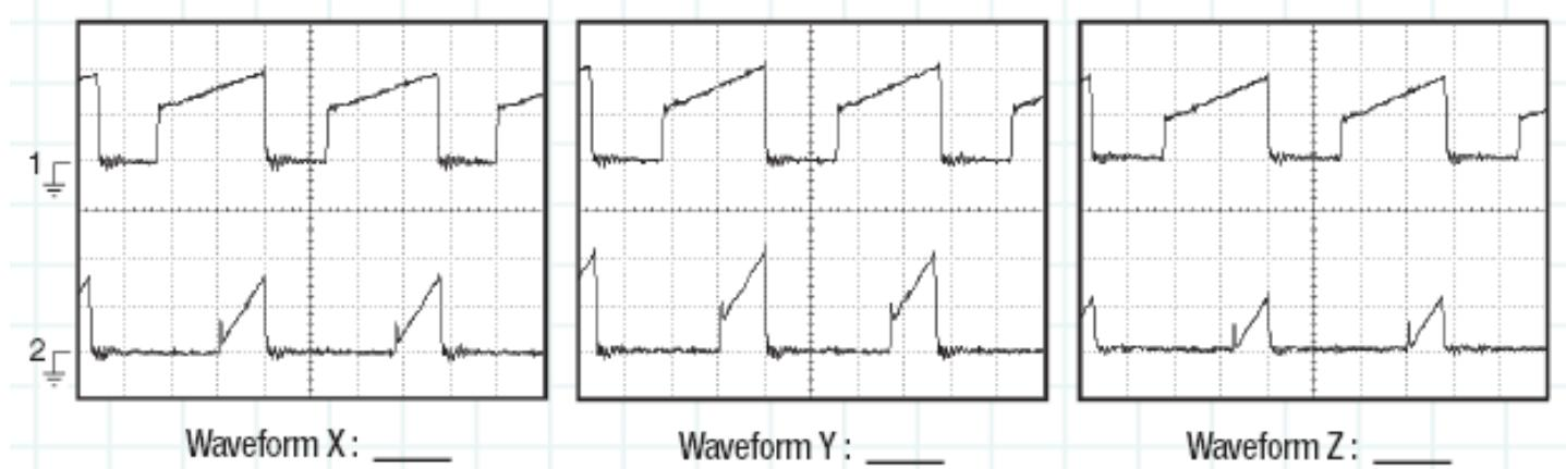
**\*Test Conditions:** Upper Trace (1)  $V_{IN} = 85$  VAC, Lower Trace (2)  $V_{IN} = 265$  VAC, both traces 0.5 A/div, 2  $\mu$ s/div
