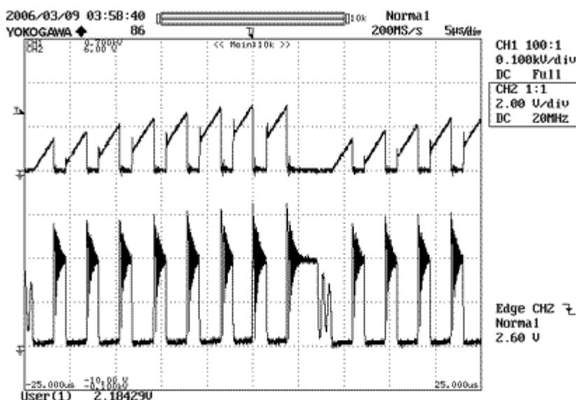
**Figure 2. Waveform shows Drain current (Top) and Drain Voltage (Bottom).**
