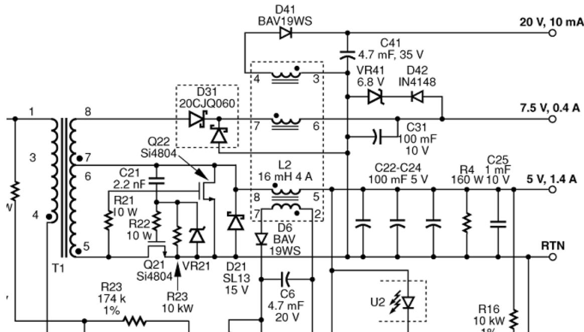
If C21 is omitted during normal operation the converter will operate normally, the positive voltage that appears across the secondary winding during the on-time of the primary switch will turn on Q21.
