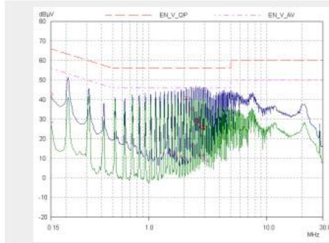
Figure 6 - *TOPSwitch* (100 kHz without jitter) Conducted EMI versus Frequency
